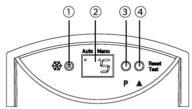
① LED red (danger of frost) ② Display screen for switching point (P) and operating mode ③ Parameter button ④ Value / Reset button
