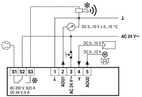
If the capillary leaks, the switch changes to the frost position. Min. active length material of capillary tube is 250 mm. Permissible cable length at 1.5 mm<sup>2</sup> diameter is max. 300 m.
