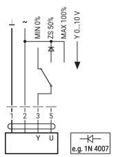
Control remotely 0...100% with positioner SG..
