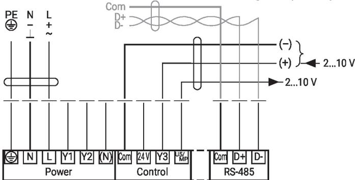
Connection of passive sensors (BACnet MS/TP / Modbus RTU)
