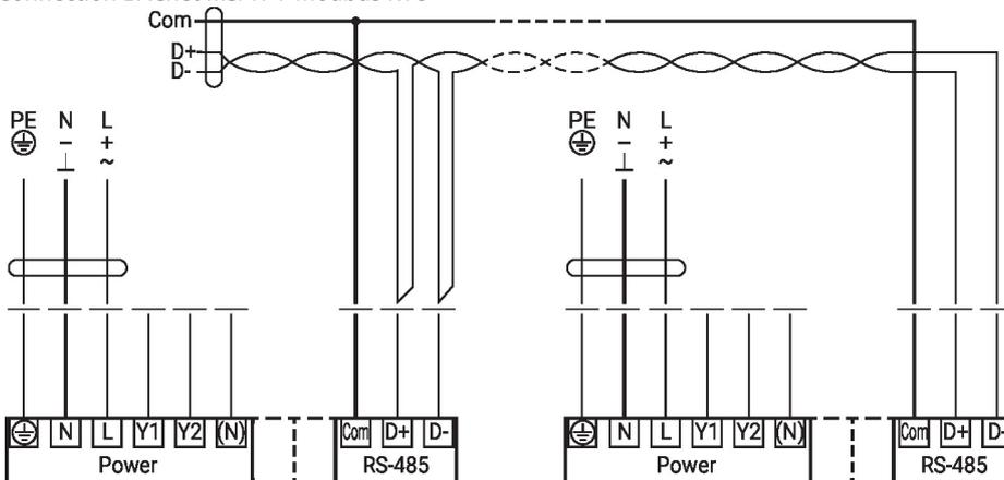
Connection BACnet MS/TP / Modbus RTU with analogue setpoint (hybrid mode)
