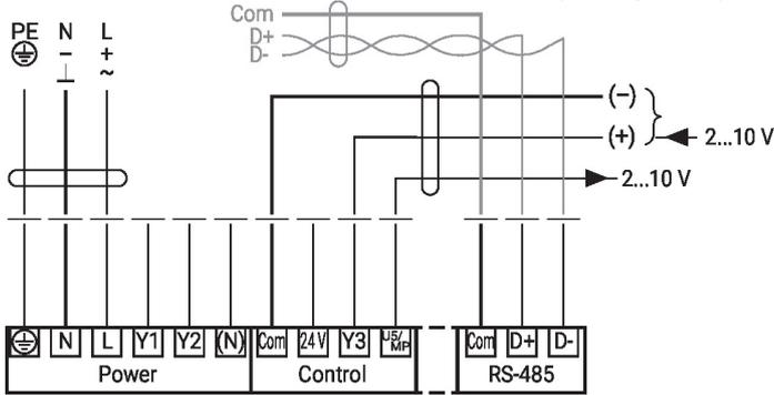
Connection of passive sensors (BACnet MS/TP / Modbus RTU)
