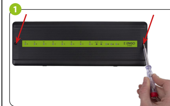
Remove the top cover of the control box
